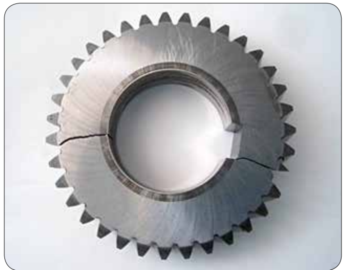
Broken single helical gear
